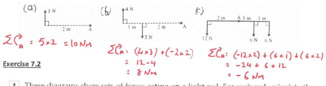
1 These diagrams show sets of forces acting on a light rod. For each rod, calculate the sum of the moments about P.
