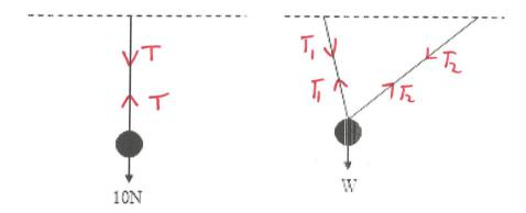
A string is tied to two points on the same level and a *smooth ring* of weight 10N which can slide freely along the string is pulled by a horizontal force, *P*. For the position of equilibrium shown in the diagram, find *P* and the tension in the string.
