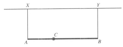
The rod AB has mass 6 kg and length 1.4 m. A particle, of mass 10 kg, is attached to the rod at point C, where AC = 0.3 m. Calculate the tension in each of the strings XA and YB. [7]
