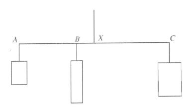
The length of the rod AC is 20 cm and the length of AB is 8 cm. The masses of the objects hanging from A, B, C are 0.1 kg, M kg, 0.4 kg respectively. The mass of the rod is 0.5 kg.
