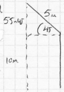
$$\text{loss in PE} = M \times 9.8 \times (10 + 5.5 \sin 45)$$
