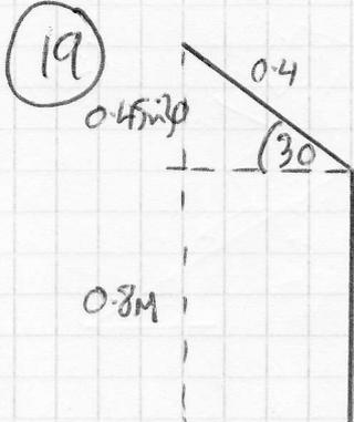
$$\text{loss in P.E.} = M \times 9.8 \times (0.8 + 0.2) = 9.8M \text{ Joules}$$
