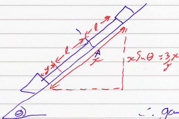
$$\text{loss in gPE} = \frac{3}{5}x \times mg = \frac{3}{5}mgx$$
