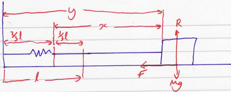
$$\text{Friction Force } F = \mu R = \mu Mg$$
