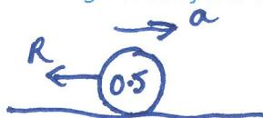
$$\begin{aligned} \text{N2L } F &= ma \\ -R &= 0.5a \quad -(1) \end{aligned}$$
