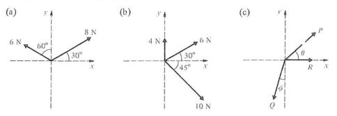
5. For each of the following systems of forces, find the sum of the components (i) in the Ox direction and (ii) in the Oy direction.
